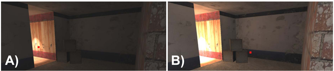
Fig. 8. Dynamic luminance adaptation based on the user's gaze point on the screen (the red square).
