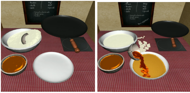
Fig. 13. New interaction possibilities: a bowl coupled to the 6DoF haptic device is used to stir the batter (left), and the same bowl pours maple syrup on the crepe (right).
